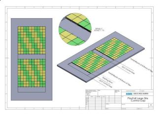
**Note:** For additional tile security, interlocking pins can also be drilled and inserted to outside perimeter material and connected to first row of tiles
