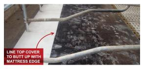
Start at the end of the roll and drill through both the top cover and mattress pad.
